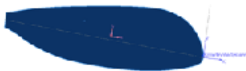
Paddle blade projected area and centroid determination.
